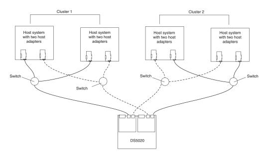
Figure 60. Example of a two-cluster configuration
